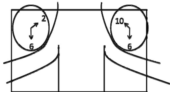
On the right, the nonthreaded portion of the screw should be directed from 6-10 O'clock. On the left, from 2-6 O'clock
