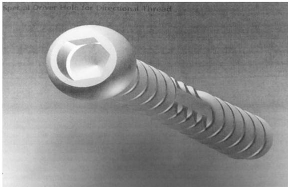
The modified pedicle screw is shown. Note how the head of the screw can only accept a driver in one configuration.
